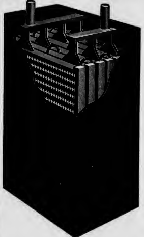
Fig. 1. View of Battery Element.
